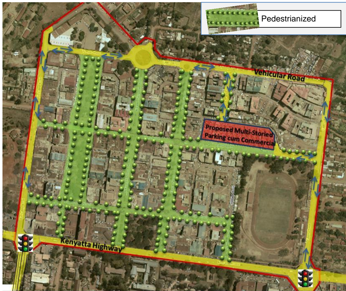
Figure 6.3: Pedestrianised roads and revised traffic circulation within CBD area
