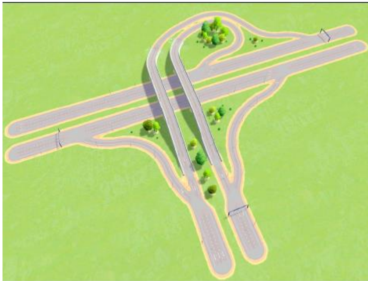
Figure 6.13: Flyover Crossing a Thoroughfare
